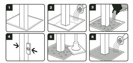
Allow 5-10 minutes for initial set to take place – following this, the post will remain in a vertical position unsupported. Postfix will achieve appreciable strength after 4 hours depending on ambient conditions but is best left overnight before attaching fence panels etc.
