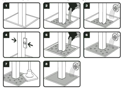
Alternatively the hole can be lined with a plastic bag or similar to stop the water draining away.
